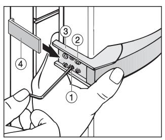
Loosely attach the handle to the opposite side of the door with the two front screws 2.
